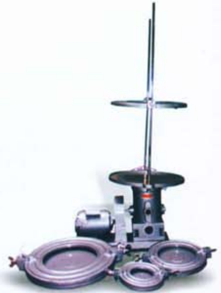
GYRATORY SIEVE SHAKER WITH ADAPTER 18" 12" 8"
