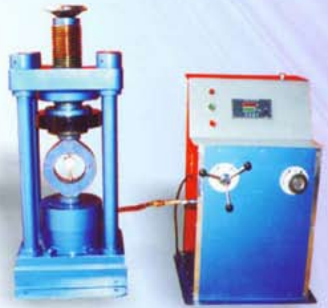
COMPRESSION TESTING MACHINE CAPACITY = 2000KN
