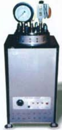
LAB. CEMENT AUTOCLAVE
