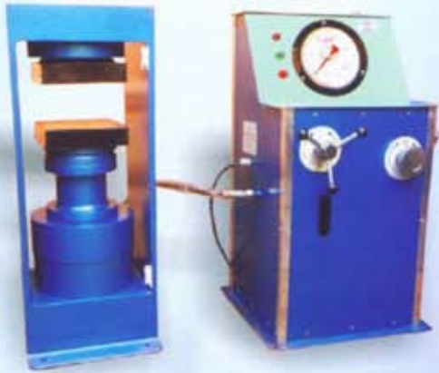
COMPRESSION TESTING MACHINE CAPACITY = 200KN SINGLE PRESSURE GAUGE
